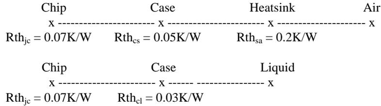
For air-cooling:  $(T_j - T_a) = (R_{th_{jc}} + R_{th_{cs}} + R_{th_{sa}}) * P_D$ , whence  $P_D = (T_j - T_a) / (R_{th_{jc}} + R_{th_{cs}} + R_{th_{sa}})$
