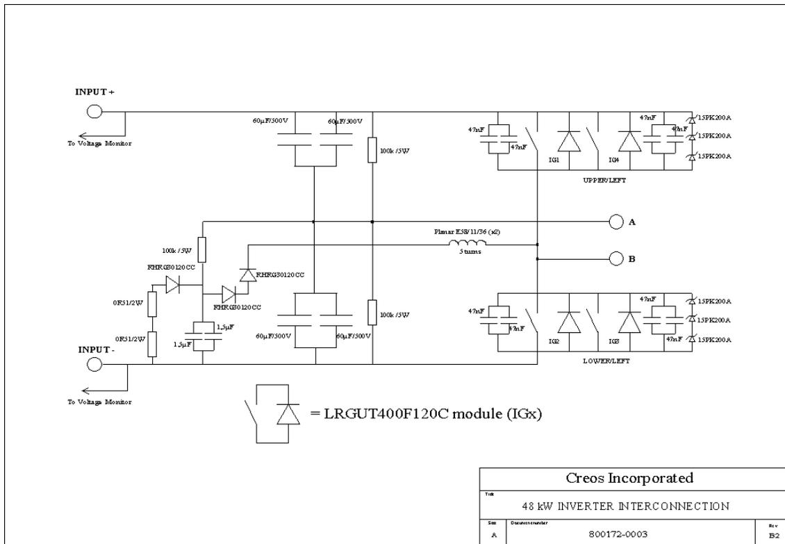
Figure 1 Inverter interconnections
