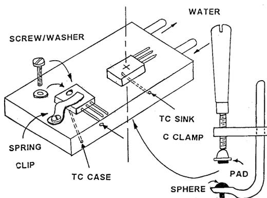
Figure 1 - Water-cooled Test Fixture
