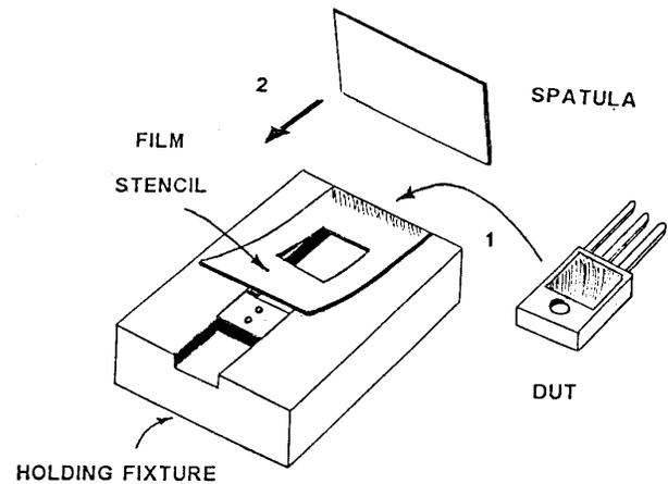
Figure 3 - HIFLOW™ Deposition Fixture
