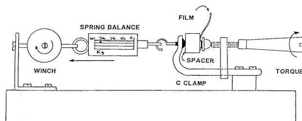
Figure 2 - Mounting Clamp Calibration
