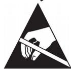
When power modules are placed in the boxes for the shipment, this symbol with the mention “Electrostatic sensitive devices, observe precautions for handling” is labeled on the boxes.
