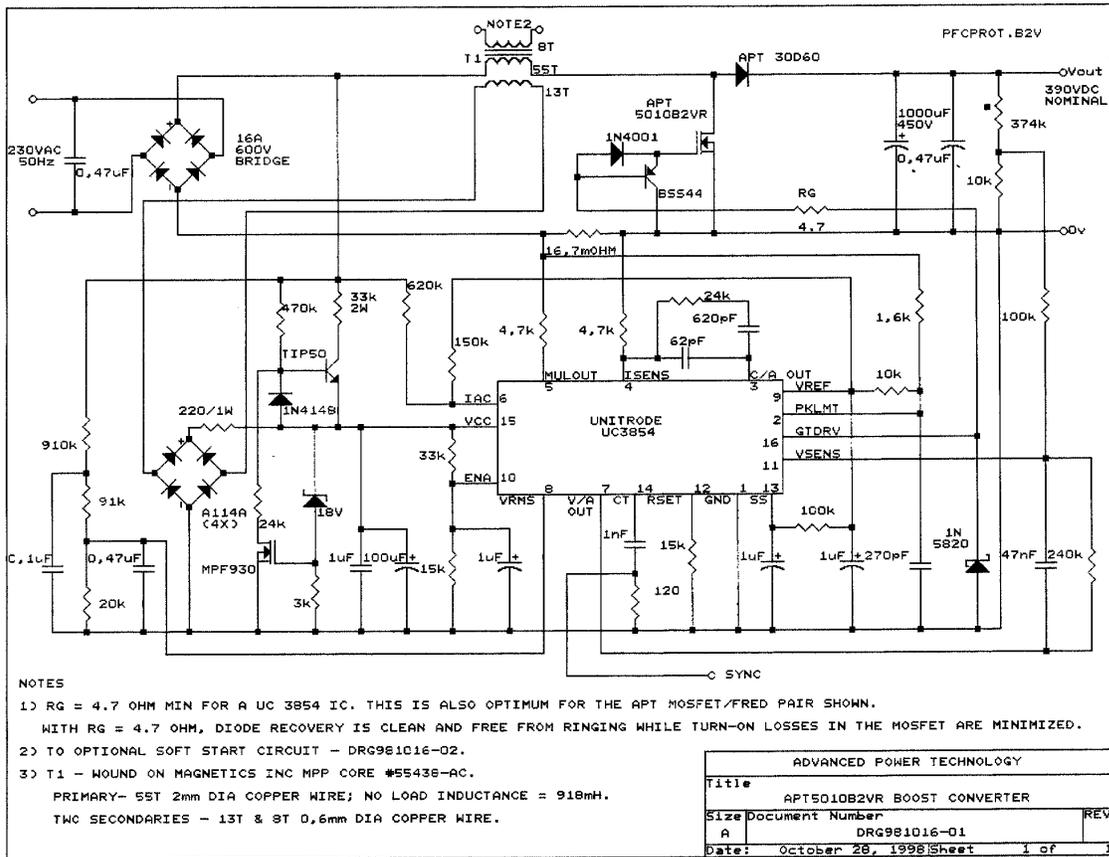
Figure 3 – Complete Boost Converter
