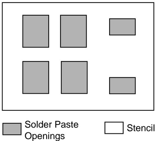
**Figure 2.** Recommended Solder Stencil Pattern for the D<sup>3</sup>PAK.
