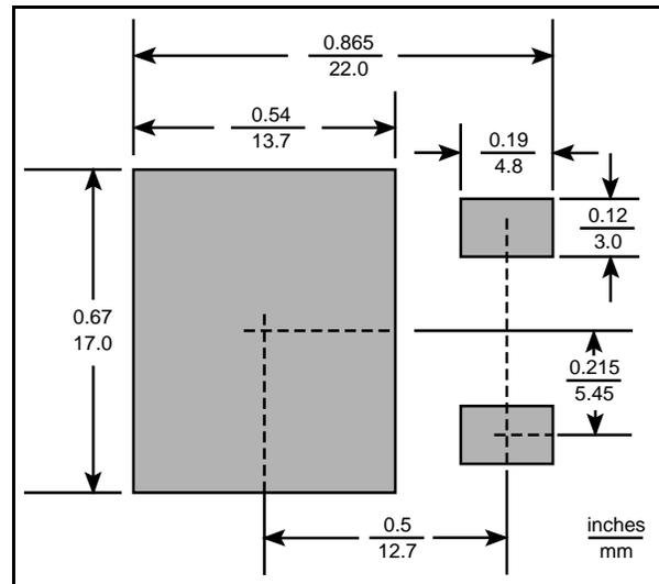
**Figure 1.** Minimum Recommended Footprint for the D<sup>3</sup>PAK.
