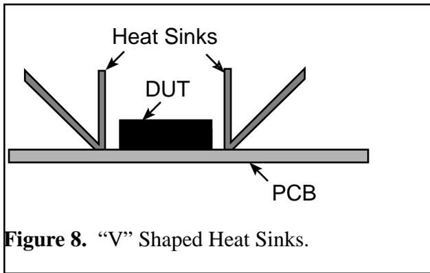
**Figure 8.** “V” Shaped Heat Sinks.
