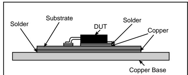
**Figure 9.** Cross Section of the D<sup>3</sup>PAK Mounted on the Substrate and Copper Base.
