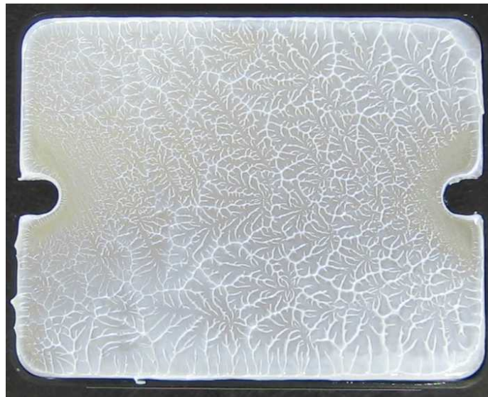
Fig 2: SP1 base plate with properly applied thermal grease after removal from heat sink.
