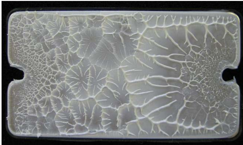
Fig 2: SP3 base plate with properly applied thermal grease after removal from heat sink.
