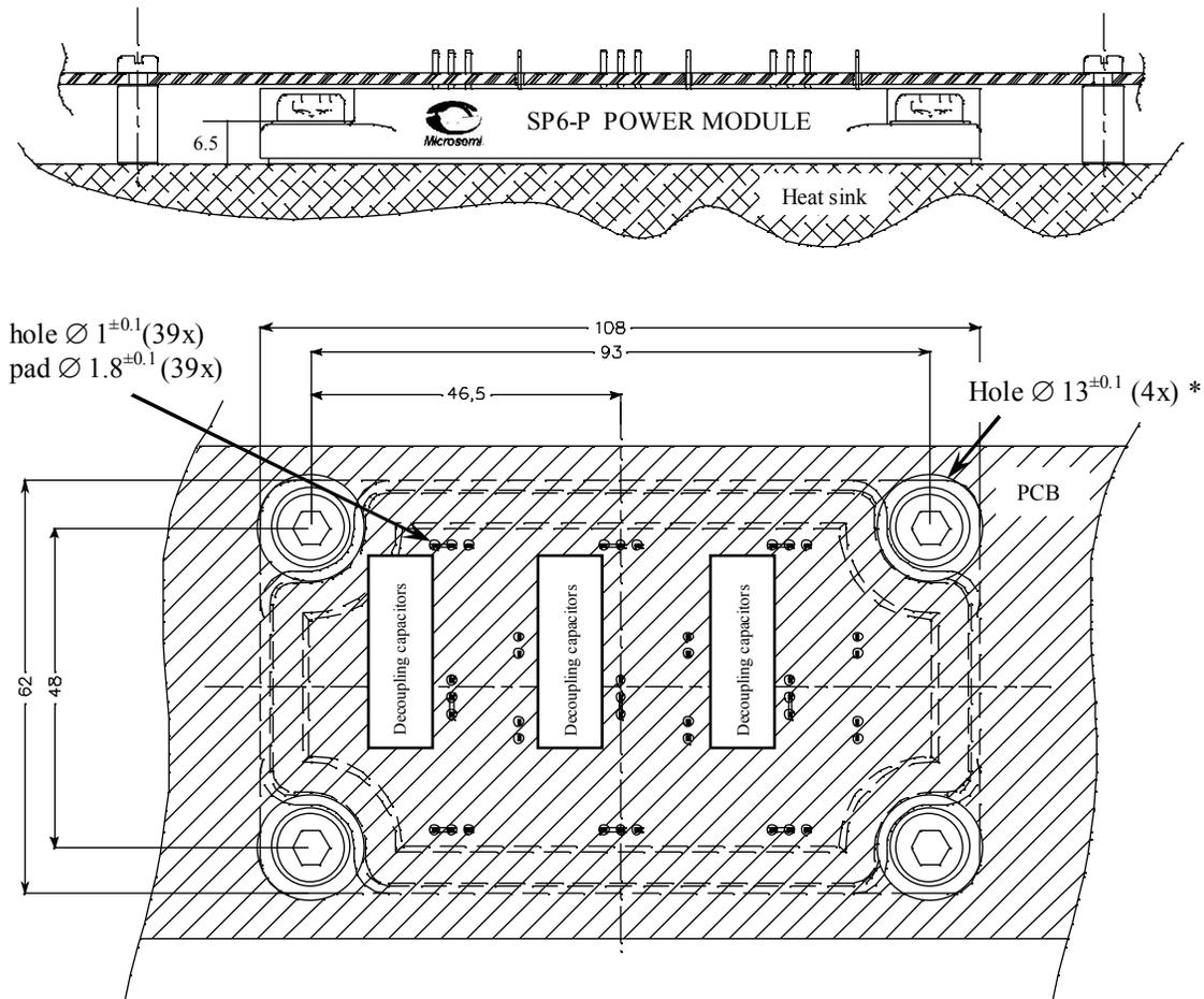
\* For spacers placed onto the mounting holes, hole diameter must be  $6.8^{±0.1}$  (4x)
