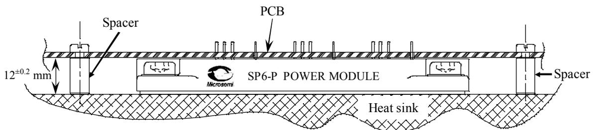
fig 1: PCB screwed onto the spacer.
