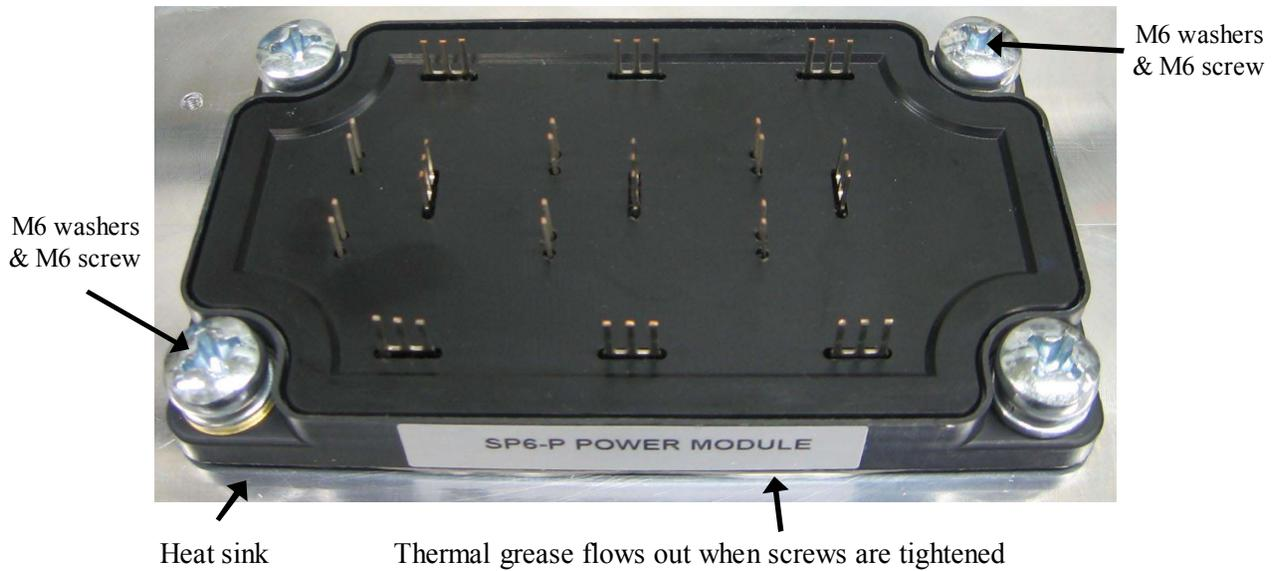
Fig 3: Proper application of thermal grease to the power module.
