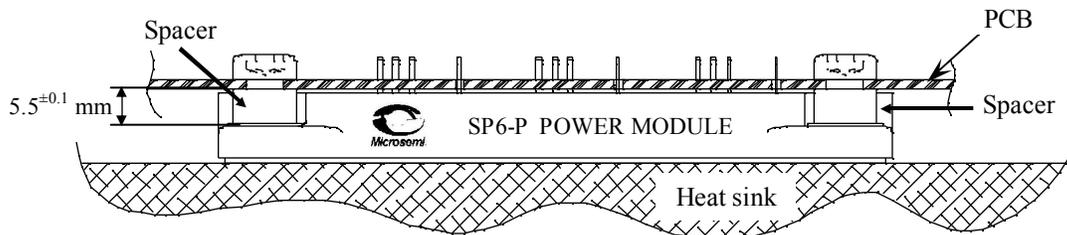
Fig 2: PCB screwed onto the mounting holes.
