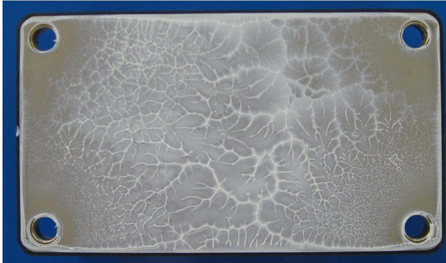
Fig 4: SP6-P base plate with properly applied thermal grease after removal from heat sink.
