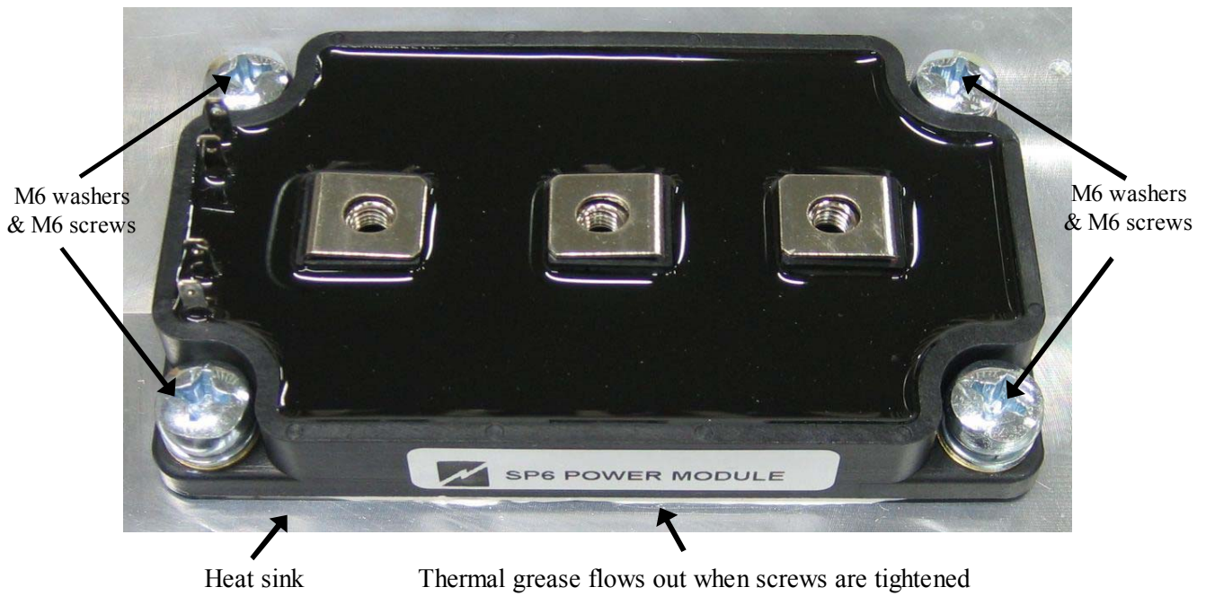
fig 1: Proper application of thermal grease to the power module.
