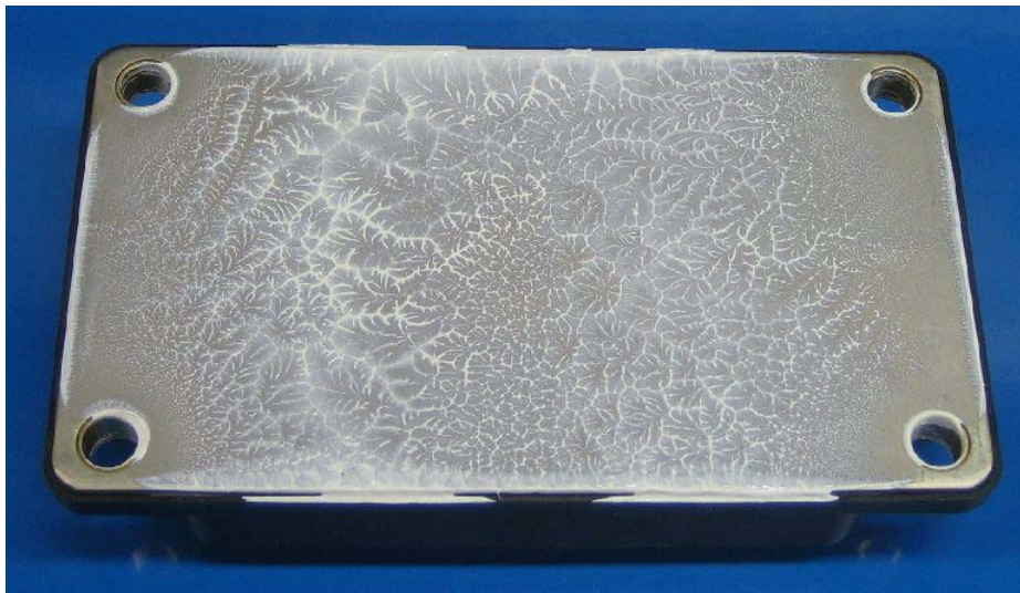
fig 2: SP6 base plate with properly applied thermal grease after removal from heat sink.
